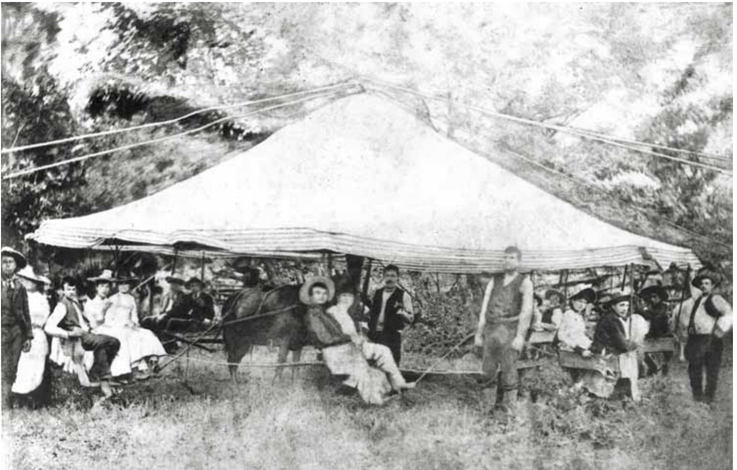
Primitive, horse-powered, suspended swing-ride with buckboard seats in Ada, OK. Photo circa 1890. Photo credit: Dell Maxwell
